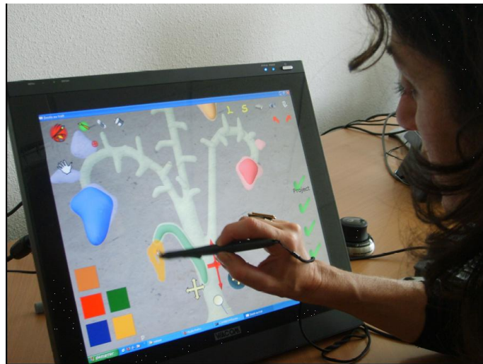
Figure 3. Azalic Studio: a free-form shape modeling tool for non-experts, based on a 2D painting metaphor.
