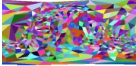
Fig. 9: The table associating a face to each (u,v) , precomputed with the hardware using an item-buffer.
