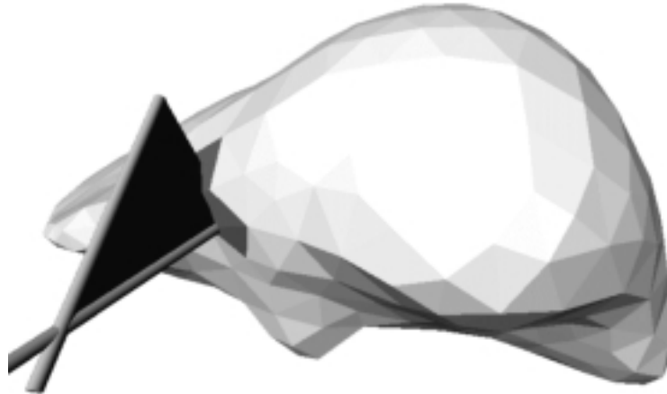
Figure 10. Dynamic collision detection, where the tool motion during a time interval is taken into account (this volume covered by the tool is visualized as a single triangle).
